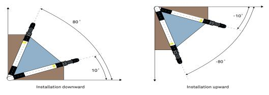
Figure 1 Recommended installation angles
