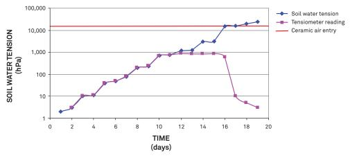
Figure 15 Tensiometer readings with tensions to -1,500 kPa
