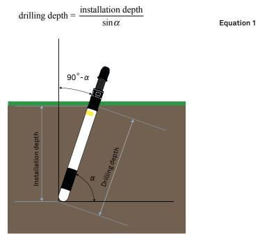
Figure 7 Drilling depth depending on installation angle
