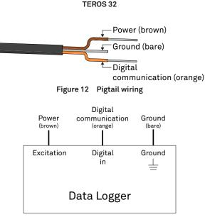
Figure 13 Wiring diagram
