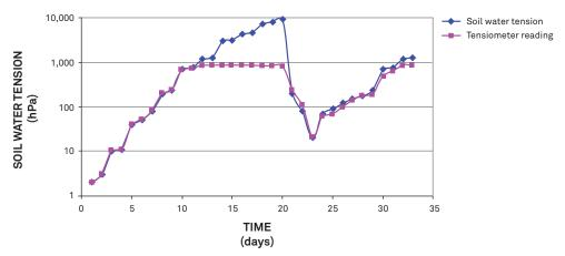
Figure 16 Tensiometer readings with tensions to -1,000 kPa
