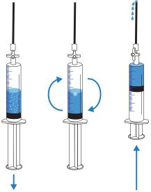
Figure 9 Degassing water in refill syringe
