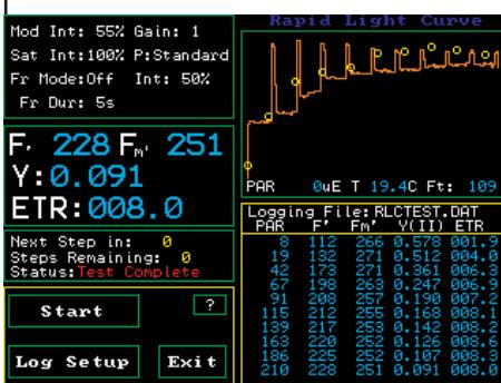
10 point experimental curve used to study light saturation characteristics in variable light conditions, such as under a canopy or aquatic work. The OS1p provides integral curve fitting software as standard.
