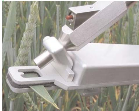
In a light adapted environment, photosynthetic Yield Y(II) varies not only with different types of plant stress, but also with light level and leaf temperature. For this reason, it is important to use a PAR clip to achieve reliable results.
