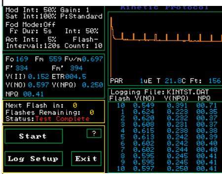
Another versatile fluorescence test, Hendrickson parameters with NPQ are provided as standard with the OS1p. Kramer Lake model parameters or Puddle model parameters may be purchased as alternative protocols at the time of manufacture.
