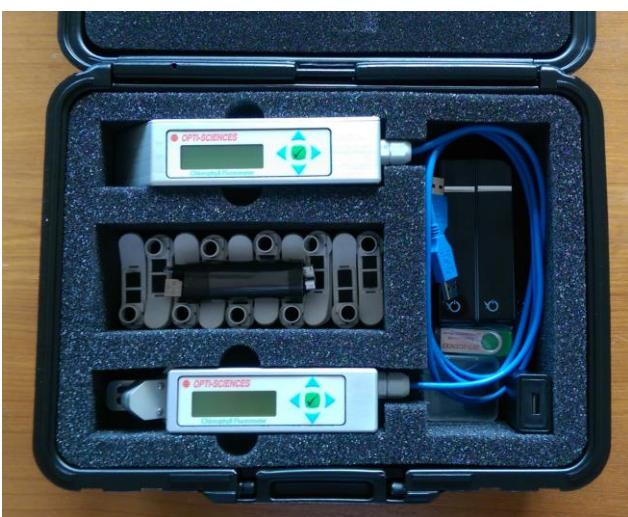
Supplied in a rigid clamshell case, the Plant Stress Kit comprises the Y(II) meter, Fv/Fm meter, 2 x Li/ion batteries, 2 x USB chargers, 2 x USB cables, 10 x dark adaption clips, 2 x absorptance calibration cards and manual on USB flash drive.
