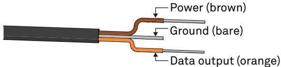
Figure 2 Pigtail wiring
