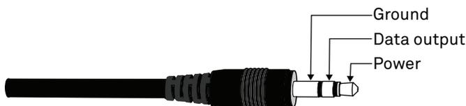
Figure 1 Stereo plug connector
