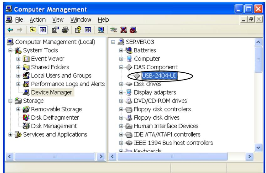
18. After installing the device drivers, open the InstaCal program from the desktop or the START menu. Before actively using the icons the serial number must be highlighted.
