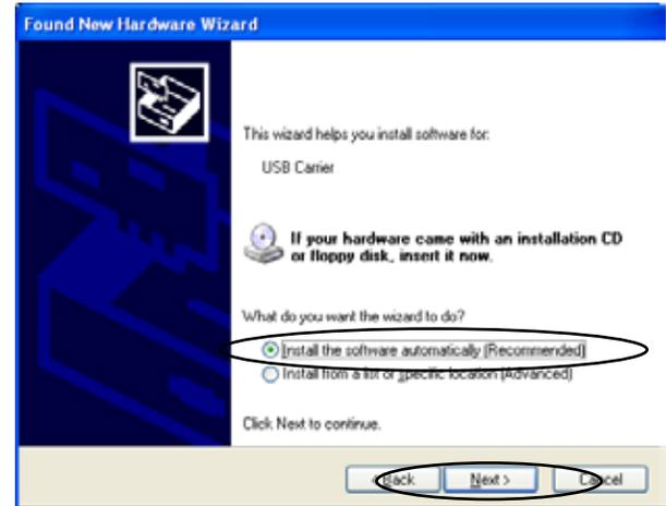
Another screen will pop up to notify you that a new device has been detected, click OK to add. The USB carrier is the generic loader for the USB2404 device.
