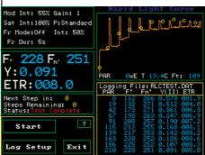
10 point experimental curve used to study light saturation characteristics in variable light conditions, such as under a canopy or aquatic work. The OS1p provides integral curve fitting software as standard.
