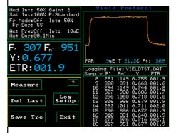
Light adapted test, the test most suited to the widest range of plant stresses and more sensitive for some plant stresses than Fv/Fm. As Photosynthetic Yield measurements can vary significantly with environmental light and temperature, it is recommended that the PAR Clip be used when making Photosynthetic Yield measurements in the field.
