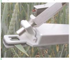
In a light adapted environment, photosynthetic Yield Y(II) varies not only with different types of plant stress, but also with light level and leaf temperature. For this reason, it is important to use a PAR clip to achieve reliable results.
