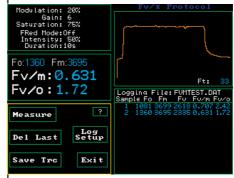
The most widely used fluorescence test requires pre-darkening of the leaf. The OS1p optimises Fv/Fm measurements by firstly automatically setting the modulated light source. Then secondly by providing a far red light option to ensure full oxidation of PSII prior to test.
