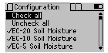
Navigate through the sensor list using 'arrows. To change the status of a sensor, highlight it and press Enter. Each sensor name you check
