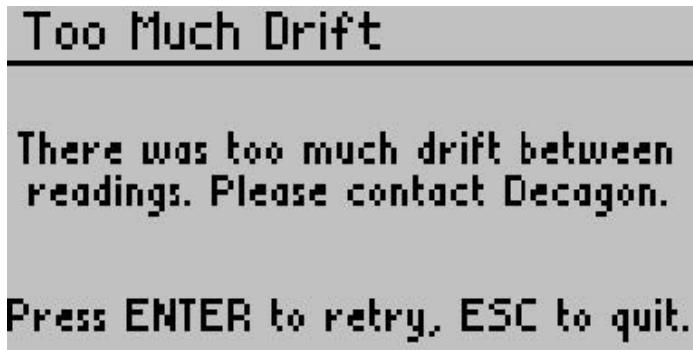
The most common problem is that thermal equilibrium has not been reached. Let the Porometer equilibrate for a few minutes and repeat the calibration process. If you still cannot achieve a good calibration, contact Decagon for help ([support@decagon.com](mailto:support@decagon.com)).
