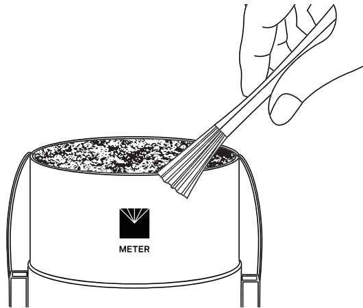
Figure 49 Fix and clean the soil sampling ring
