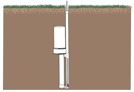
Figure 1 G3 Drain Gauge below root zone
