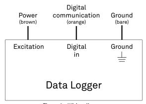
Figure 4 Wiring diagram
