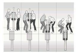
Lower the G3 into the Installation Hole
