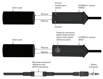
Figure 6 HYDROS 21 sensor
