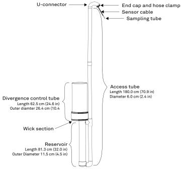
Figure 5 G3 Drain Gauge
