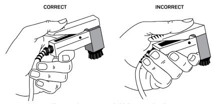
Figure 4 Correct way to hold the sensor head
