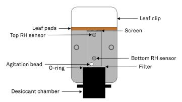
Figure 26 Sensor head internal components
