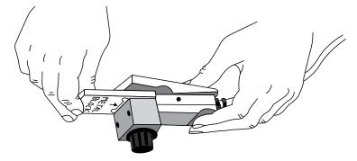
Figure 51 Sensor head on calibration plate
