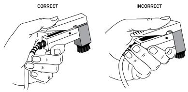
Figure 43 Holding the sensor head
