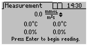
Figure 7 Measurement tab before beginning a reading
