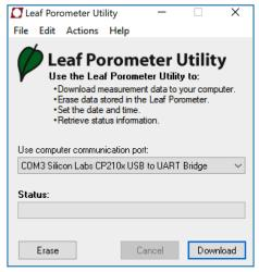
Figure 19 Leaf Porometer Utility main window
