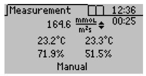
Figure 35 Measurement tab in Manual mode
