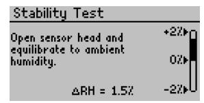
Figure 48 Stability Test screen
