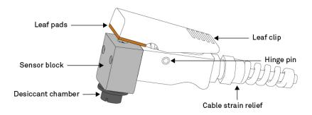
Figure 25 Sensor head external components
