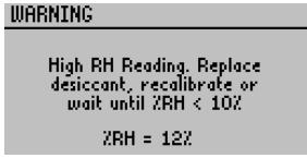
Figure 9 Warning screen for high RH reading
