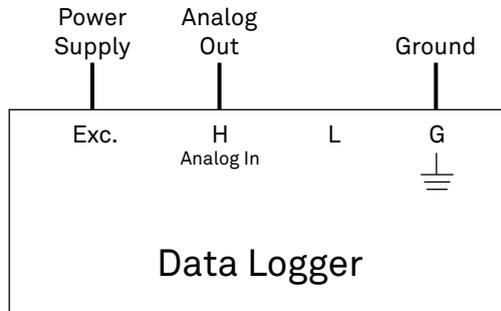
Figure 3 Wiring diagram
