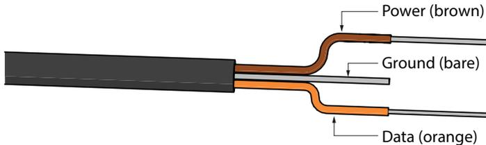
Figure 2 Pigtail wiring
