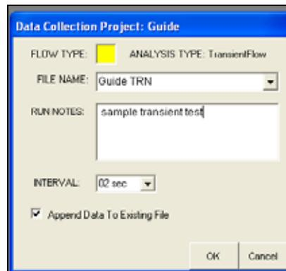
5. Confirm HCFM CAT pressure at 0 kPa according to pressure gauge. Click **Start** and a new window will pop up. Enter a **FILE NAME** and comments, select **INTERVAL** and click **OK** button. Once you have selected a file name data collection will automatically begin. As soon as the first points appears on the graph start the pressurization.
