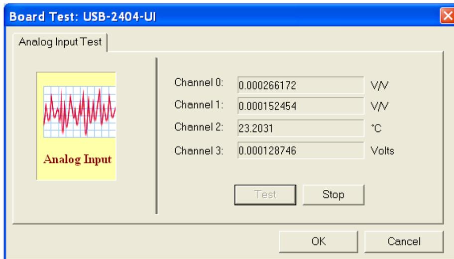
The voltages at zero pressure should be as shown, less than .004 V (<1 micro V) at maximum pressure (560 kPa) applied, the voltage is about .008 V, see the calibration section for details on other pressure/ voltage comparisons. A valid temperature in degrees C, should appear as well.
