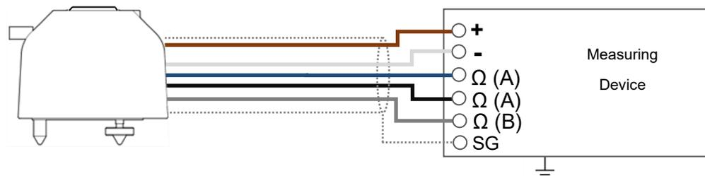
Figure 5-2. How to Connect MS-20
