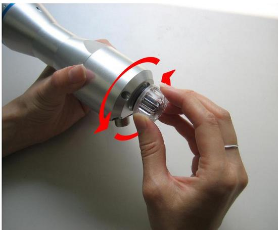
1) Turn the drying cartridge in anti-clockwise. No tools are required.
