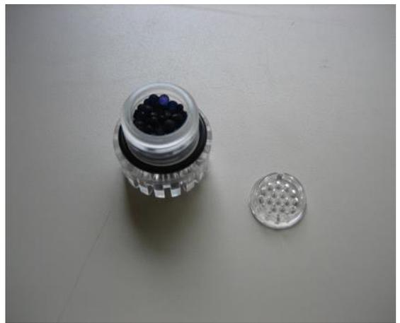
4) Exchange the desiccant then put the inner lid back on the cartridge. Place the drying cartridge back on the MS-57 body and secure it gently.
