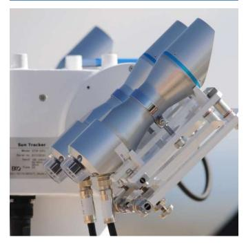
The MS-57 Pyrheliometer is an essential instrument, often used for solar assessment, research, concentrated photovoltaic applications and solar monitoring. Mounted on a sun tracker, the MS-57 with its ultra-fast <0.2s response, unique characteristics and superior design, ensure best in class accuracy, speed, and reliability whatever your application.
