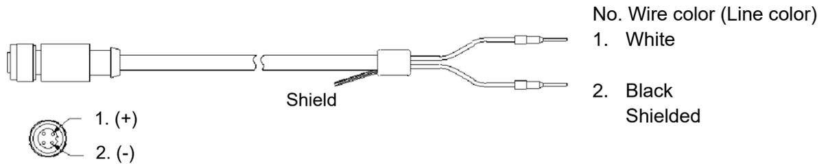
Figure 7-2. Output-Cable [MS-60]
