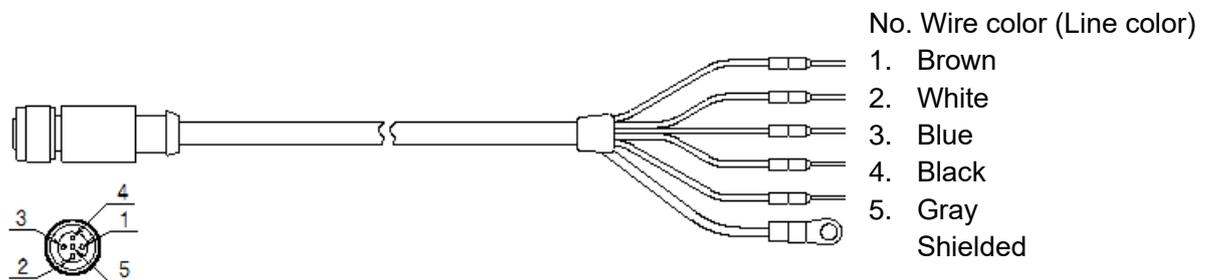
Figure 7-3. Output-Cable [MS-60S]
