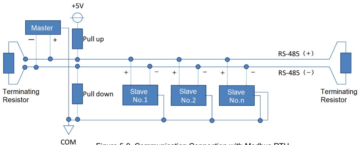
Figure 5-9. Communication Connection with Modbus RTU
