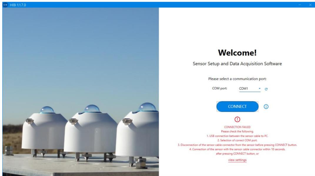
Figure A3-8. CONNECTION FAILED
