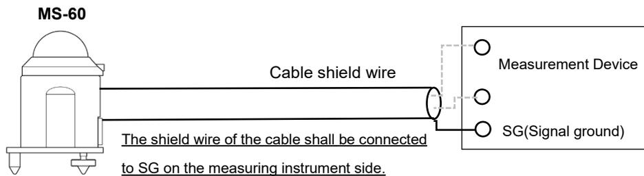
Figure 5-3A. MS-60 shield wire connection method
