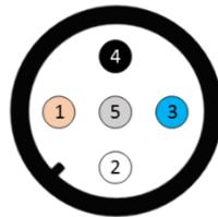
Figure 5-13. Connector pin number of MS-60S
