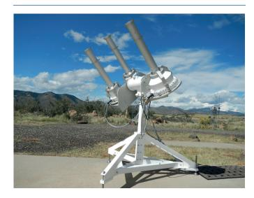
The WISER I is a research-grade configuration, combining the MS-711 and MS-712 Spectroradiometers. A reference tool for UV-VIS-NIR measurements, the WISER I covers the spectral range from 300nm to 1700nm and is designed for meteorological, plant science, photovoltaic research, and material analysis applications that require the highest standards of accuracy and reliability.
