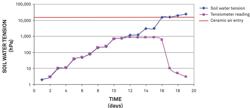
Figure 15 Tensiometer readings with tensions to -1,500 kPa
