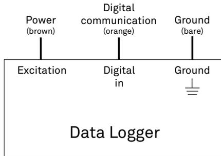
Figure 13 Wiring diagram
