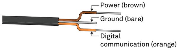
Figure 12 Pigtail wiring
