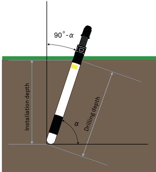
Figure 7 Drilling depth depending on installation angle
