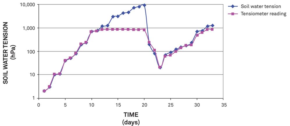
Figure 16 Tensiometer readings with tensions to  $-1,000$  kPa
