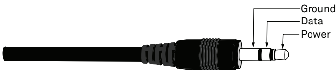
Figure 1 3.5-mm stereo plug connector wiring
