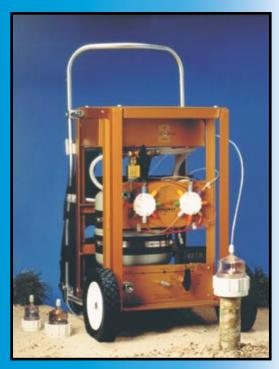
The complete HPFM-C system is field portable with detachable wheels and backpack. Operating the HPFM is Easy
