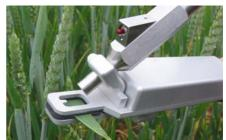
Photosynthetic Yield Y(II) varies not only with different types of plant stress, but also with light and temperature. It is therefore important to use the supplied PAR clip to achieve reliable results.
