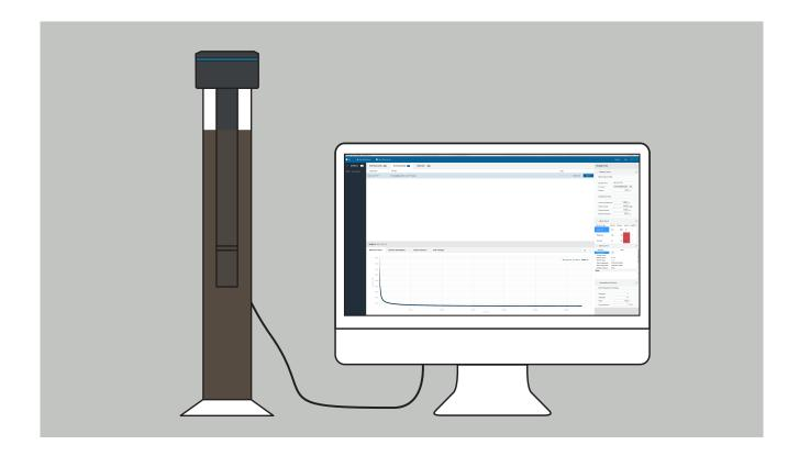
From now on, PARIO Control will record a measurement data triple (time, pressure, temperature) each 10 sec and depicts the recorded data graphically. The status line of the running measurement is moved automatically from the list "Preparation" to the tab "In Progress".
