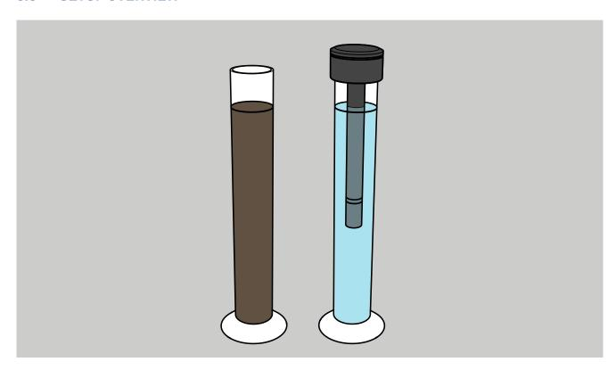
For performing a sedimentation analysis with PARIO® you need to place one cylinder with the prepared soil sample and the other one with distilled room tempered water on a plane surface. Insert the PARIO® in the distilled water for temperature equilibration and connect it to the computer.
