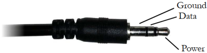
Figure 8: 3.5 mm Stereo Plug Wiring
