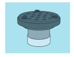
When the saturation is completed, close the soil sample with a lid, turn the whole system upside down and put it in a pan. (If there is only one soil sample in the saturation pan you can leave it there)
