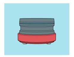
Turn the sample under water rightside up. Remove the other lid and put the blue marked (bigger) part of the adapter air free with the marking line upwards on top of the soil sampling ring.
