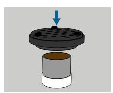
Flip the adapter and place it on top of the soil sampling ring.
