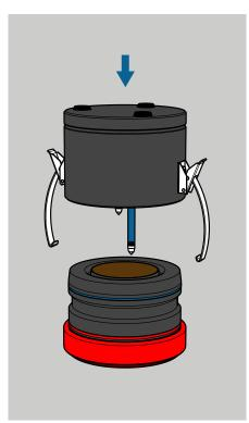
Put the refilled HYPROP® (for instructions about the preparation of the HYPROP® please read the HYPROP® manual) on top of the soil sample, turn the system upside down, remove the red sealing and close the HYPROP® clips.
