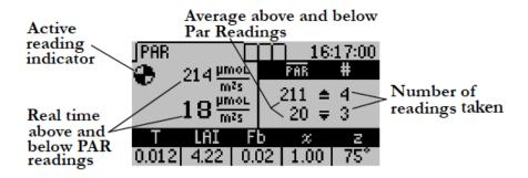
LP-80 updates and displays the current calculated Tau  $(\tau)$ , LAI value, beam fraction  $(F_b)$ , leaf distribution parameter  $(\chi)$  and zenith angle (z) values are updated and displayed at the bottom of the screen with each subsequent below canopy PAR measurement. If the external sensor is attached and you press an up or down arrow, the LP-80 records both above and below canopy readings.
