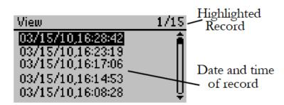
You can scroll between different readings using the up and down arrows. To view detailed data from a selected record, press the ENTER key while highlighting the record. The LP-80 displays the stored data.
