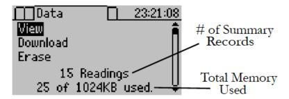
You can view summary records and their relevant data, download the data to your computer terminal for analysis, or erase the data memory from the Data screen. To select one of the options in this menu, scroll to the desired item and press the ENTER key.
