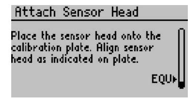
With the moist filter paper in place, slide the calibration plate into the sensor head, making sure you have oriented the side of the plate marked "Metal Block" toward the aluminum block side of the sensor head.
