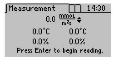
At the top of the screen is the stomatal conductance number at left, and the currently selected unit of measurement at right. Below are two columns of numbers. The left is the sensor closest to the leaf, and the right is the sensor farthest from the leaf. Each column has the temperature of that sensor, and its percent humidity. The Leaf Porometer uses these to calculate the stomatal conductance value.
