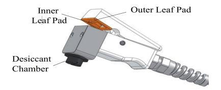
Figure 1: Sensor Head External Components
