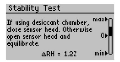
Once the sensor readings stabilize and are confirmed to be within 2% relative humidity of each other, the calibration routine automatically advances to the next screen. If the sensors do not equilibrate to similar humidity values, check for water on the sensor head. If no water is found, then the sensors may have been chemically contaminated or be otherwise malfunctioning. If this case occurs, you should recondition the sensors. Section 8.3 has more details on reconditioning the sensors.
