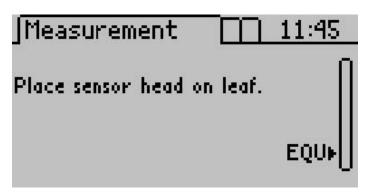
4. The reading will begin once the sensor head is placed on a leaf, and it detects a conductance value greater than 5 mmol m<sup>-2</sup> s<sup>-1</sup>. A progress bar will also indicate the reading is underway.
