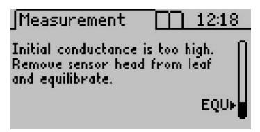
If you see the screen above, close the clip and allow the sensor to equilibrate. If an agitation bead is in place shake the sensor head briskly in a vertical orientation to more quickly equilibrate.
