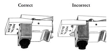
Figure 4: Correct Calibration Plate Installation
