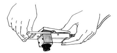
Figure 3: Calibration Plate Installation
