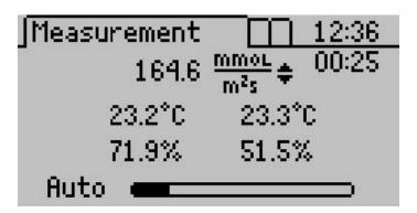
7. Once the 30 second measurement has been completed, the Porometer displays the final conductance. You may save or discard your data. The "Saving Data" portion of Section 5.2 has further instructions.
