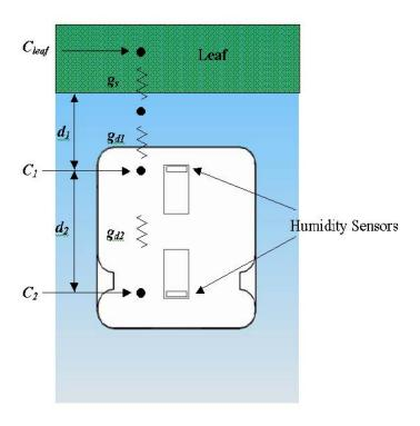
Figure 15: Leaf Porometer Function
