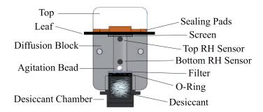
Figure 5: Sensor Head Diagram
