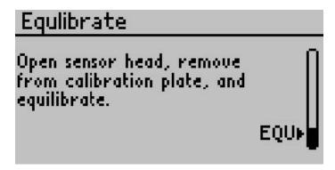
Remove the sensor head from the calibration plate and close the clip. If you are using the agitation bead, shake the sensor head to mix the air in diffusion path to speed up the equilibration process. As the sensors come to equilibrium, you should see the indicator bar move closer to the "EQU" line. Once the sensors have equilibrated, the Attach Sensor Head screen will automatically reappear and steps 8-10 can be repeated.
