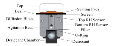
Figure 7: Sensor Block and Desiccant Chamber Components
