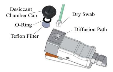
Figure 16: Desiccant Chamber Assembly
