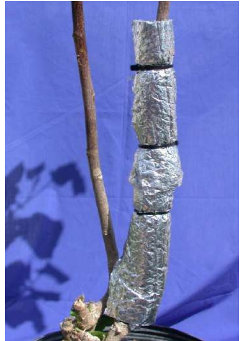
Figure 4.7 - Bubble foil Shield installation over sensor
