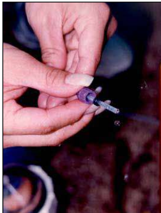
Photo 14 Connecting the “Clear” tubing w/2 larger “o” rings
