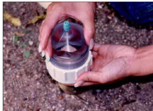
Photo 12 Tightening the Coupling
