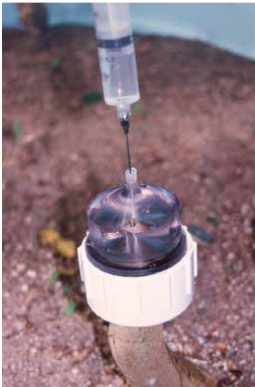
Photo 13 Removing Air from the Coupling
