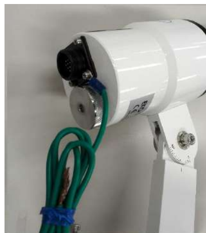
Figure 5-5. Grounding Cable attached to the sensor Main Unit
